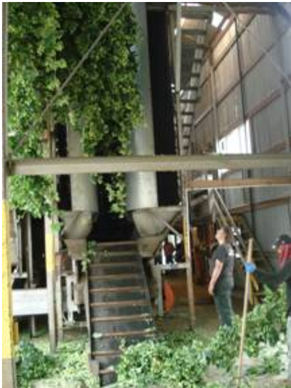
The hops bines are then hooked onto the picker machine, which “picks” the hop flowers from the bines.
